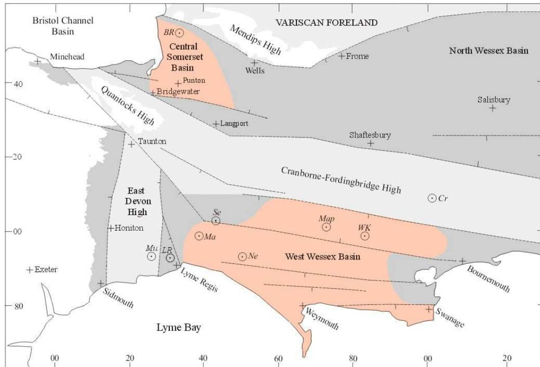
**Figure 4.** Relationship of the distribution of thick halite deposits in the Mercia Mudstone Group in south-west England to major faults in the Variscan basement. Eastern area after Harvey and Stewart (1998).
